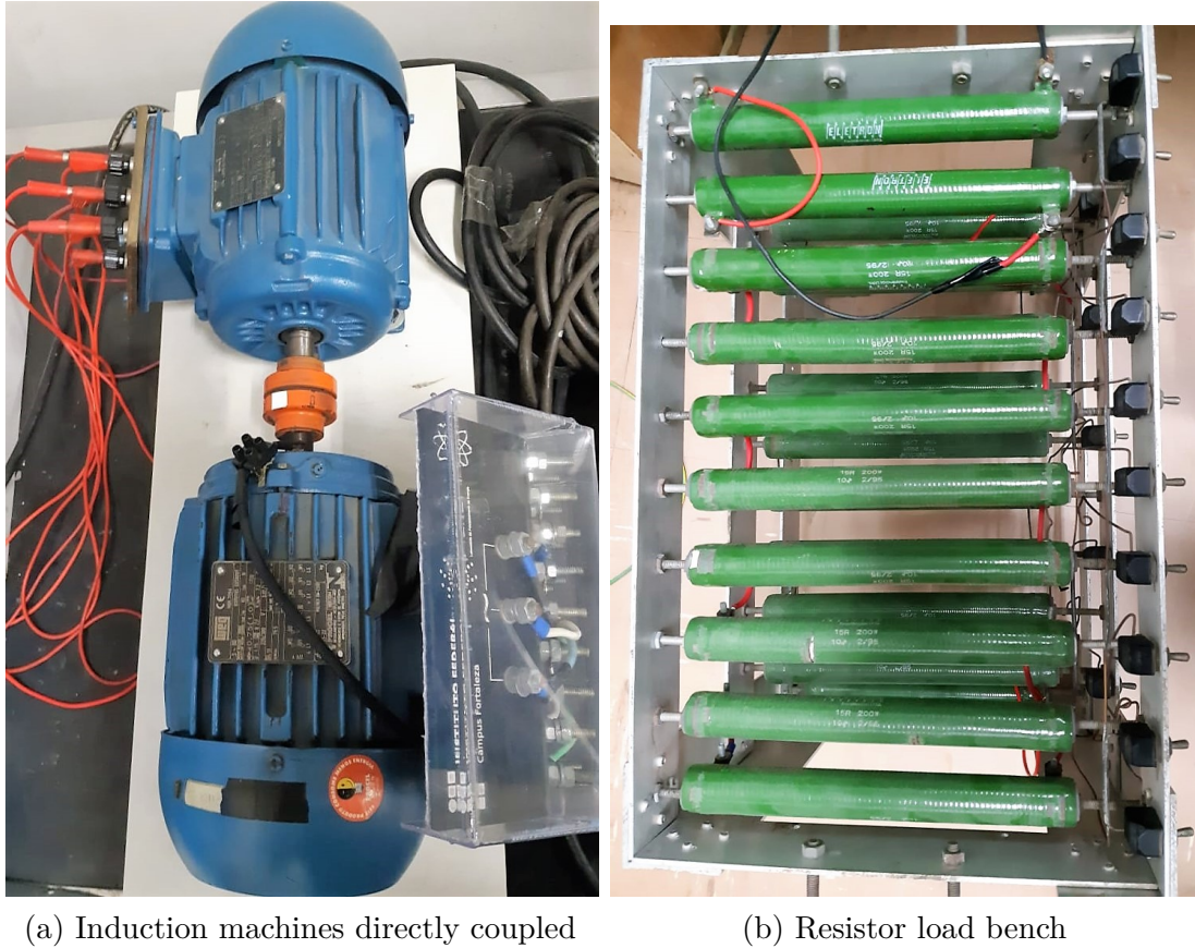
Figure 16 – Equipment used to emulate mechanical load
