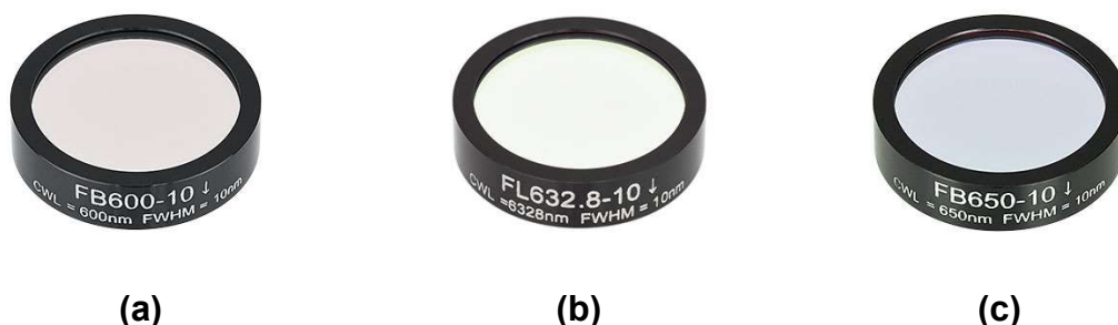
Figura 30 – Filtros passa-banda. (a) 600 nm; (b) 632,8 nm; (c) 650 nm
