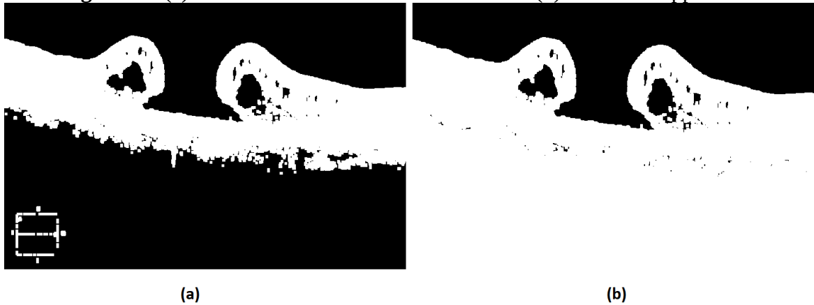
Figure 34: (a) A series of erosions and dilations and (b) Flood Fill application
